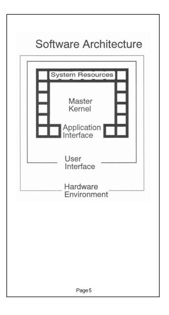
**Master Kernel** contains analysis algorithms, proprietary techniques, etc. It draws upon a library of **System Resources:** file management systems, sorting programs, graphic processing, etc. This is all embedded in the **Applications Interface**, yielding an external style appropriate to the intended application, such as word processors (WordPerfect, WordStar, Microsoft Word, etc.) and spreadsheet programs (Lotus, Excel, etc.).
